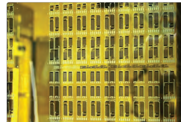
Reel-to-reel printed resistors for sensor applications
