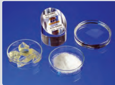
Development of optical devices – from the monomer, prepolymer and polymer to the athermal all-polymer AWG
