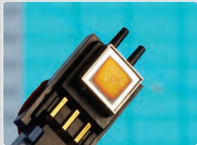
Silicon micropump in plastic housing
