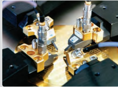
4-port measuring equipment for RF characterization of coupled structures
