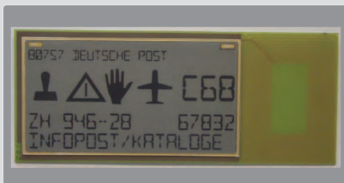
Smart label (electronic information carrier - Passive RFID system - 2nd generation bistable display)
